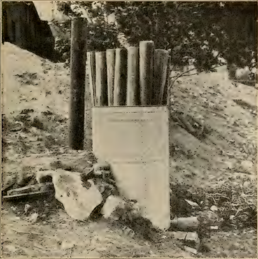
FIG. 4. SINGLE TANK HEATED BY DIRECT FIRE
