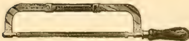
Fig. 16.—Hack saw. The thread for tightening the blade is located in the handle.
