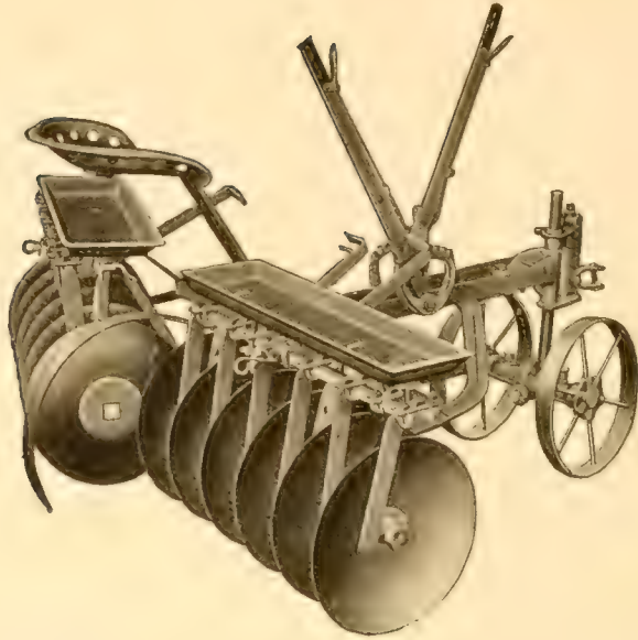
Fig. 7.—The Disk Harrow. Note the pan in which weights can be placed if necessary. The two gangs can be set at different angles for side hill disking.
