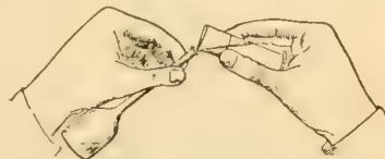
Fig. 5.—In pouring acid into the test bottle, incline the bottle a little, to avoid spilling acid on the hand.
