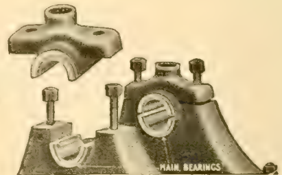
Fig. 17. Main crank bearings, horizontal Engine.
