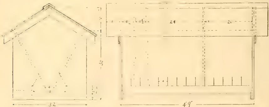
Fig. 9.—Working Plans of a Double Outdoor Hopper. Courtesy of the New York Experiment Station, Cornell.
