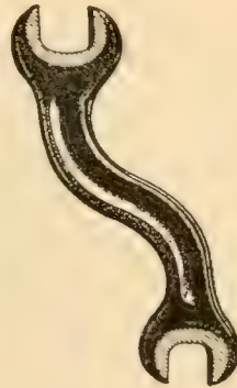
Fig. 9.—Solid, or S, wrench.
