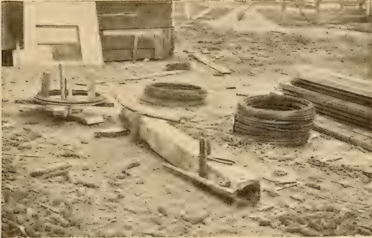
Fig. 25.—Showing method of straightening wire by drawing through a bent pipe. Courtesy of the Iowa Experiment Station
