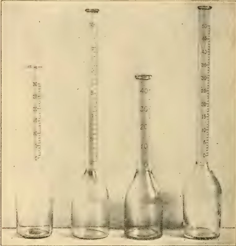
Fig. 17.—Type of cream bottle which is widely used. The smallest graduation should be 0.5 per cent. The 6-inch bottles are most common, as the 9-inch sizes require a special centrifuge.
