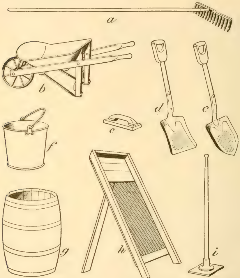
Fig. 13.—Tools Used in Making Concrete On the Farm; a, Rake; b, Wheelbarrow; c, Wooden Float; d, Square-Nosed Shovel; e, Round-Nosed Shovel; f, Bucket; g, Water Barrel; h, Gravel Screen; i, Tamper.
