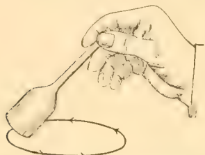
Fig. 6.—To mix the acid and milk whirl the bottle in a circle until the contents are of a uniform brown color.
