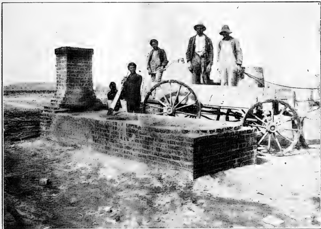
FIG. 4.—A simple form of lime-sulphur cooking plant similar to those shown in Figure 3 but with practically triple the capacity. Three kettles afford means for continuous operation, one being used for heating water and the others for cooking the concentrate. An undesirable feature is that the finished product must be dipped out.
