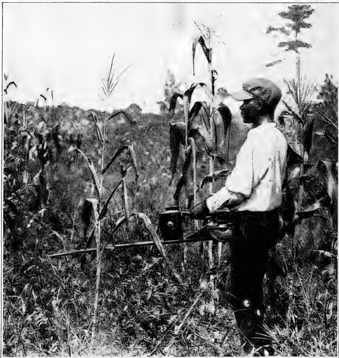
FIG. 12.—Hand duster which may be used in applying calcium arsenate or lead arsenate to forage plants infested with corn earworms.
