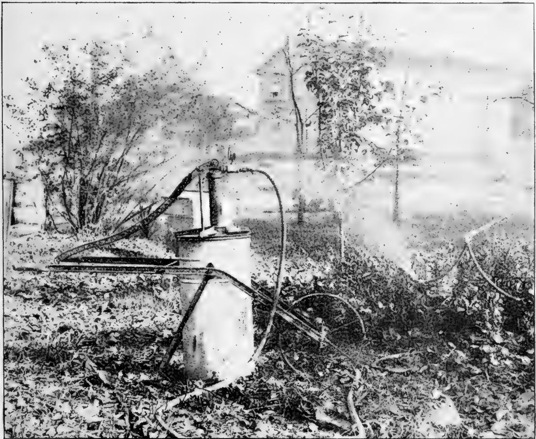
FIG. 13.—Good type of wheelbarrow sprayer effective for small patches. This sprayer holds 12 gallons, and 150 pounds pressure can be kept up when 2 nozzles are used.
