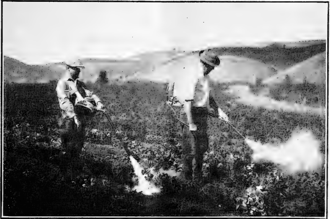
FIG. 14.—Two types of hand-operated dusters used in an infested pea field: At left, fan type; at right, bellows type.
