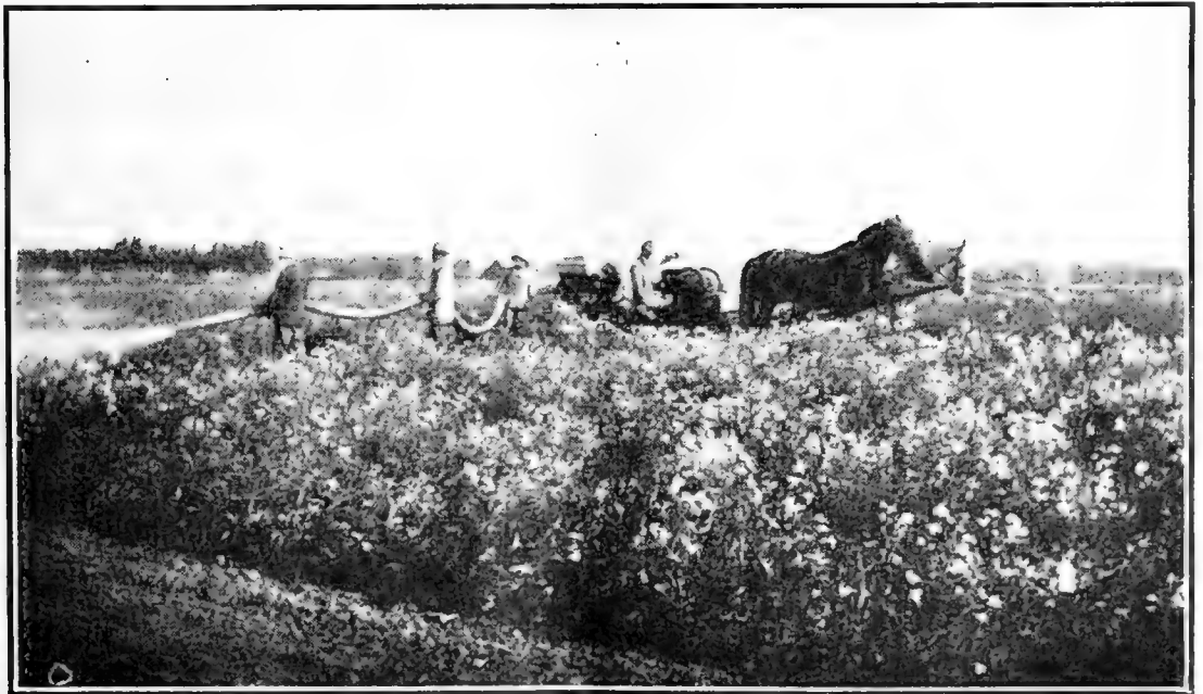
FIG. 10.—Power-operated duster with single discharge pipe, used in field of sweet peas when plants are too large to permit driving down the rows.
