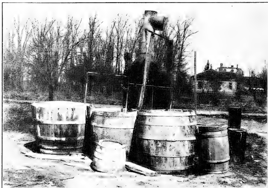
FIG. 17.—It is undesirable to use lime-sulphur cooking vessels of different sizes. Such an arrangement necessitates the weighing of different amounts of materials for each container.
