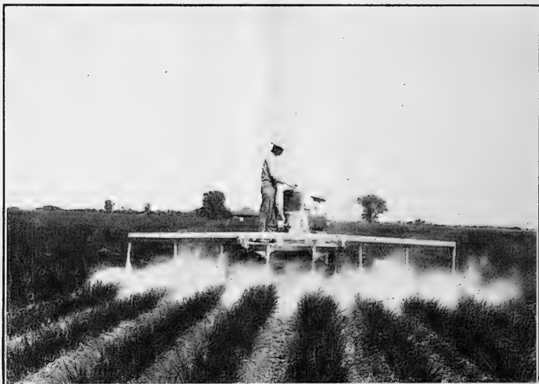
FIG. 13.—Large power-operated duster for applying dust to combat onion thrips; rear view.
