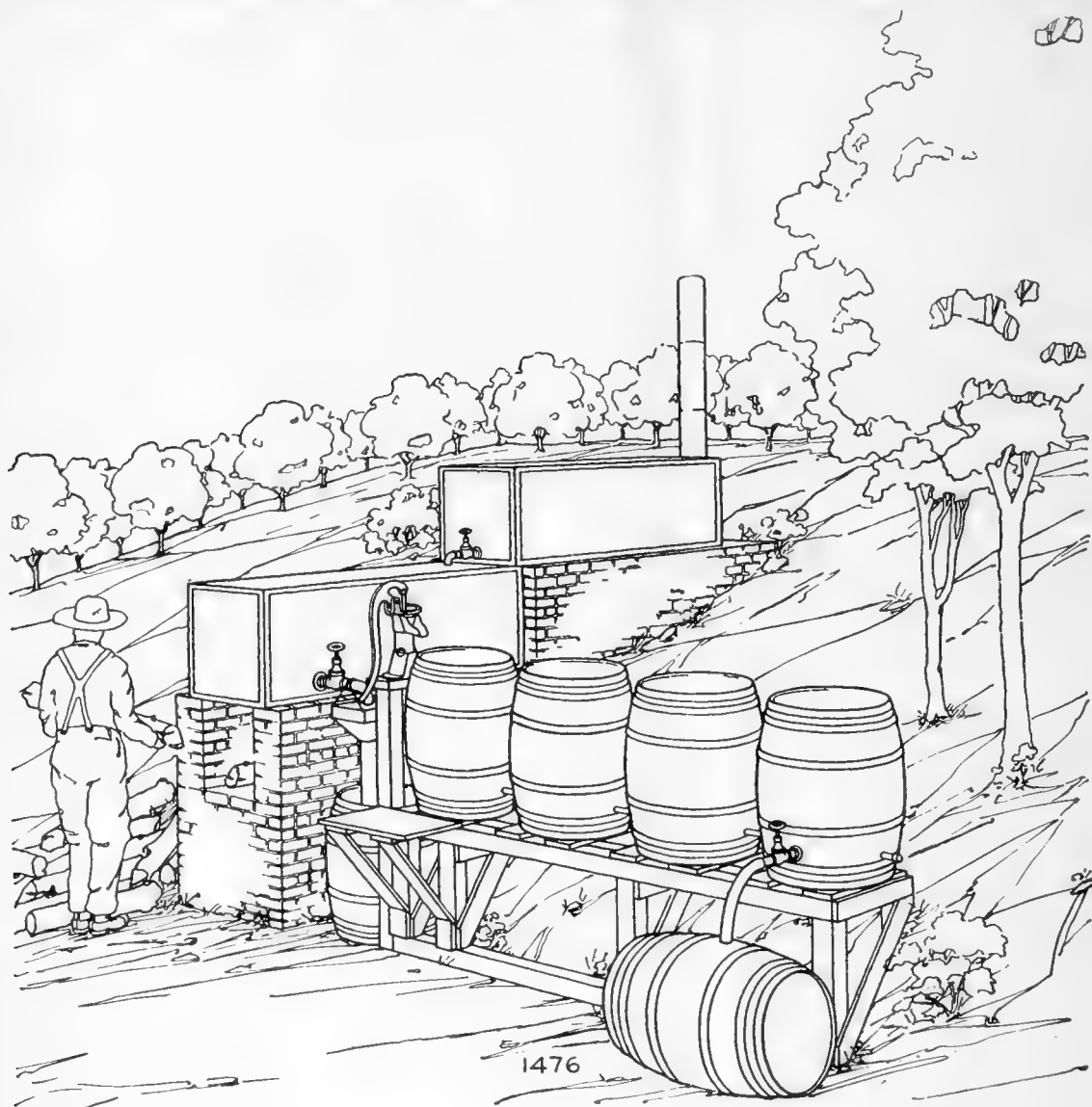
FIG. 5.—Hillside furnace type of lime-sulphur cooking plant.
