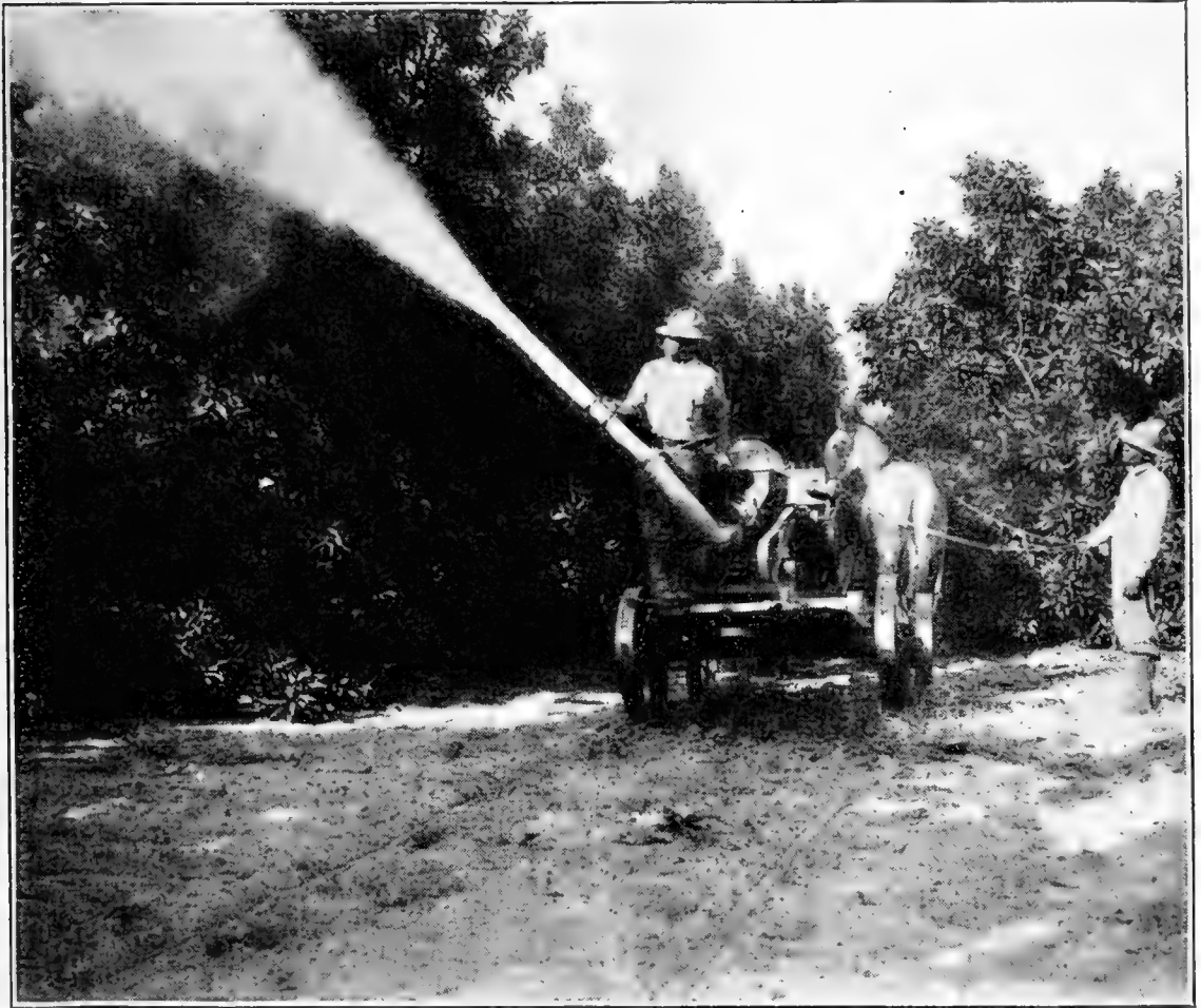
FIG. 21.—Power duster in operation against red spider on avocado trees.
