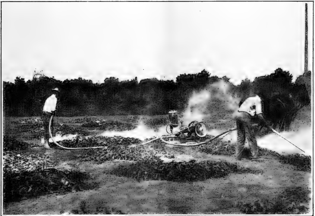
FIG. 4.—Power-operated fan duster used with success in a badly infested melon field.
