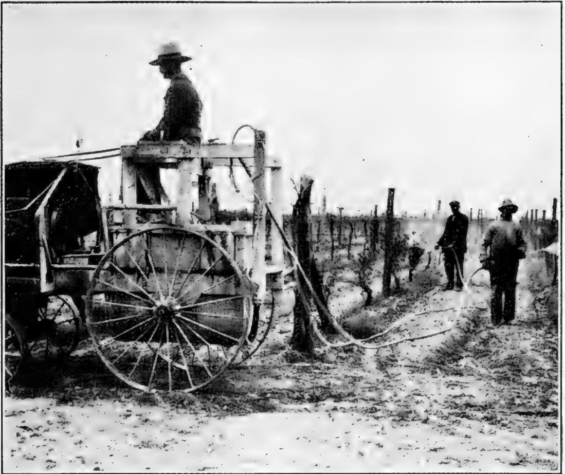
FIG 76.—Gasoline power grape sprayer, illustrating the so-called trailer method of applying the spray.
