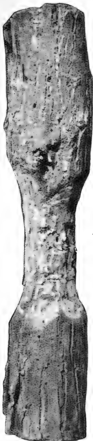
FIG. 4.—Section of mesquite stick after four months work by smaller powder-post grubs, showing depth to which sapwood is eaten. The small holes in the bark are made by the adults which have emerged.
