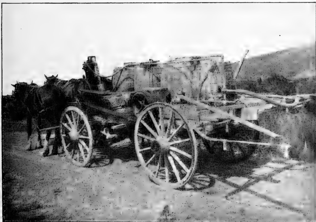
FIG. 6.—A homemade spray outfit. No part of this equipment was originally designed for spraying. Even the nozzles were homemade. In convenience and utility it is equal to any spray machinery manufactured.
