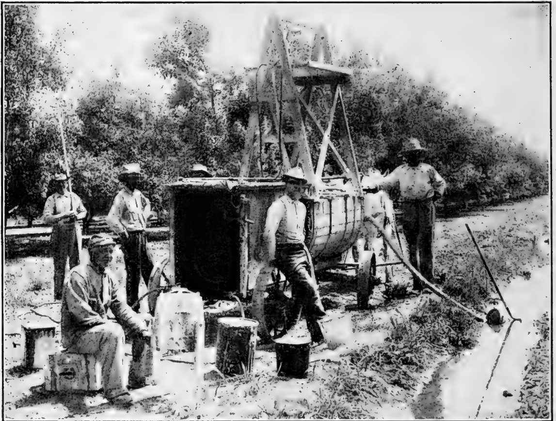
FIG. 15.—Gasoline-power spraying outfit with carpenter's horse type of tower and rotary pump tank filler. (Quaintance and Siegler.)
