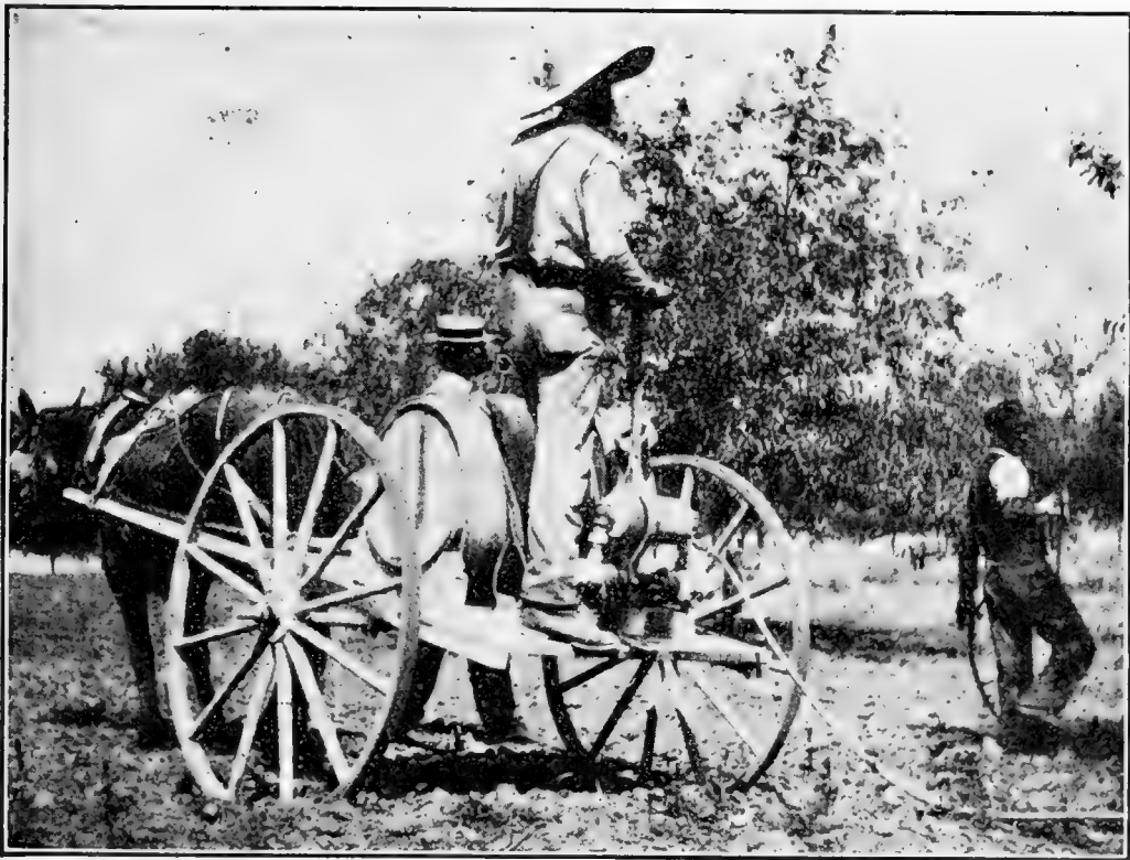
FIG. 10.—Double-action hand pump for spraying home grounds or in the small community. (Quaintance and Siegler.)
