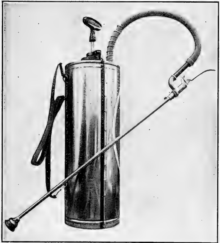
FIG. 8.—Compressed-air sprayer for small spraying operations; no pumping is required while spraying. (Quaintance and Siegler.)
