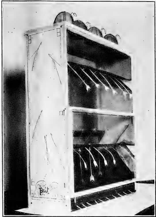
Fig. 8.—The Hodge flytrap, showing where the flies enter. (After Hodge.)
