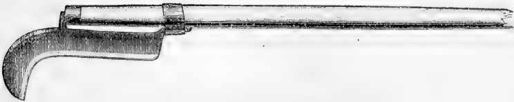
FIG. 519.—LONG-HANDLE BUSH HOOK.
