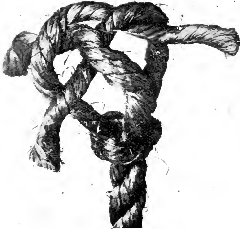
Fig. 11.—The Wall Knot below and the crown above, showing position of the three strands before hauling taut.
