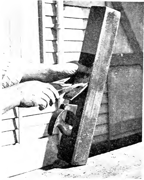
Fig. 9.—Inserting the Iron and Wedge in the Try and Jack Planes.
