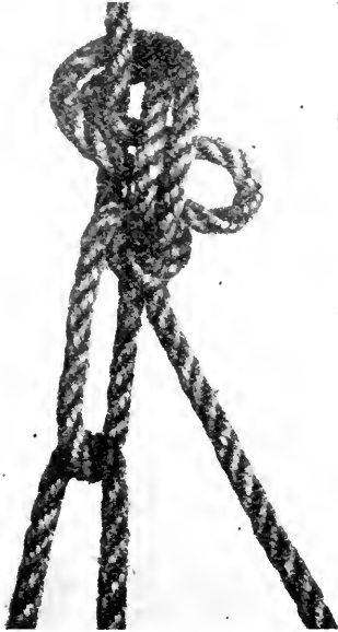
Fig. 31.—The Hay Knot made so as to prevent any chance of slipping.
