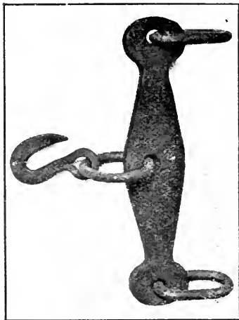
Fig. 6.—An appliance for obtaining a correct line of draught when leading harness is used in ploughing.
