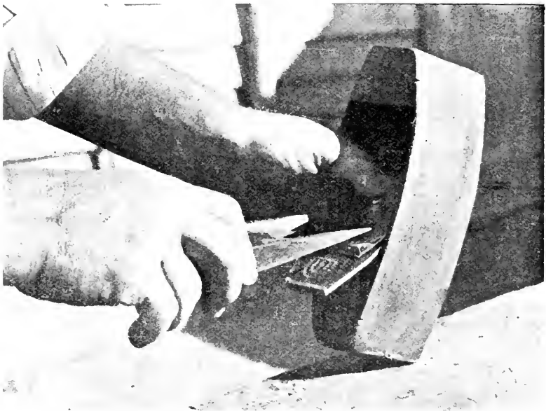
Fig. 13.—Inserting the Iron and Wedge in the Smoother.
