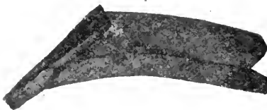
Fig. 17.—The lay ready for welding.
