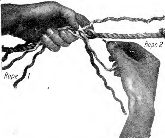
Fig. 3.—Short Splice. The position of the hands, placing the first strand of Rope 1 under Rope 2.
