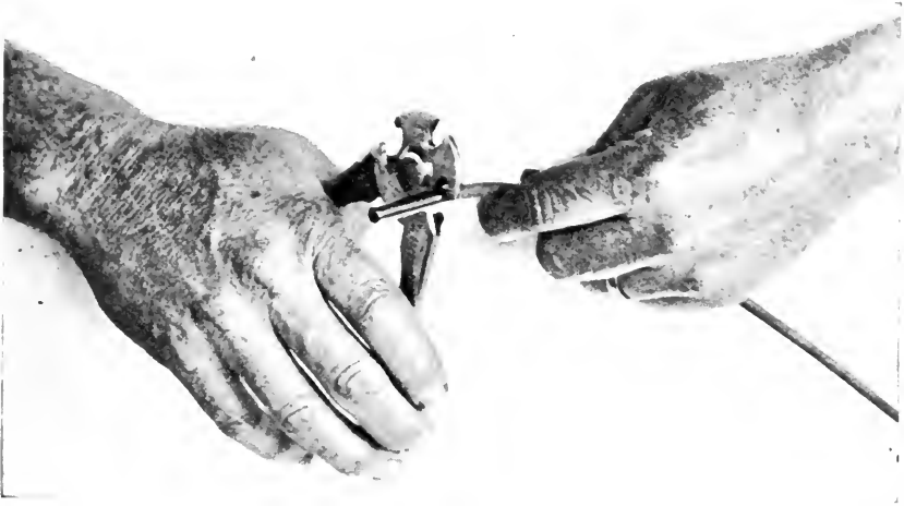
Fig. 4.—Crimping the cap on the fuse.
