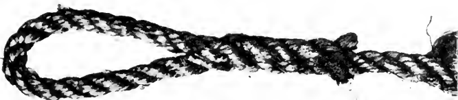
Fig. 9.—The Eye Splice finished. Not tapered.
