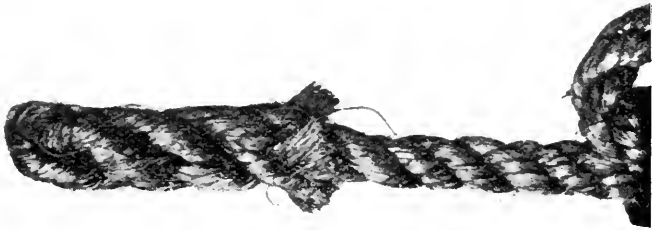
Fig. 12.—The crown made by itself, and the strands spliced back a short distance down the rope (not tapered).
