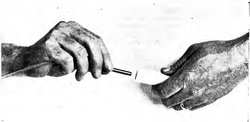
Fig. 6.—Inserting the capped fuse in the gelignite.
