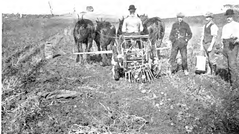
One form of Potato Digger. Rear view, showing tubers leaving revolving apron and falling on riddle.
