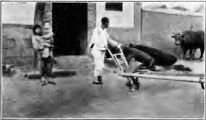
FIG. 114. - Double row seed-drill, just returning from the fields to the village home.
