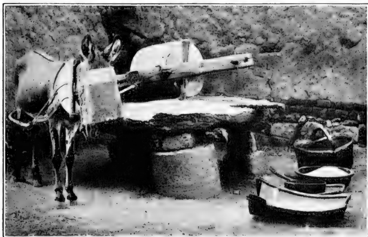
FIG. 51. — Stone mill in common use for grinding beans and various kinds of grain.
