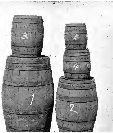
1, \frac{1}{2} LEAGUER, OR ABOUT 63 IMPERIAL GALLONS; 2, AN AUM, OR 32 GALLONS; 3, \frac{1}{2} AUM, OR 15 GALLONS; 4, AN ANKER, OR 7\frac{1}{2} GALLONS; 5, A KEG OR \frac{1}{2} ANKER, 4 GALLONS. (All in round numbers.)
