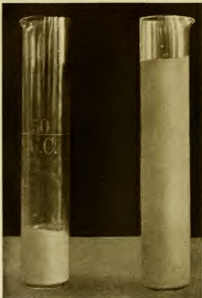
17. WHERE EFFICIENCY IS THE DETERMINING FACTOR For each quart of cream left by the milk by a good separator shallow setting yields less
