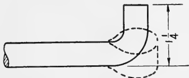
FIG. 190. Upsetting for clevis.
