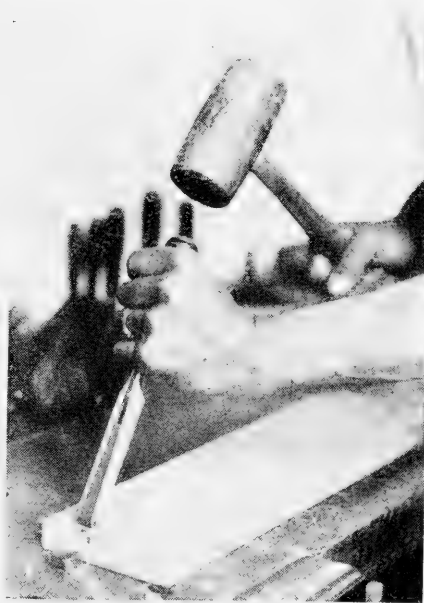
FIG. 92. Chiseling across the grain.
