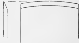
FIG. 58. Shape of cutting edge for jack plane.
