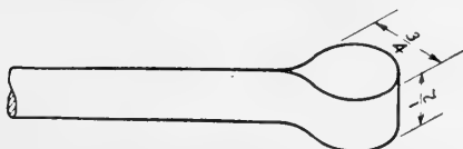
FIG. 192. Appearance of finished job of upsetting.
