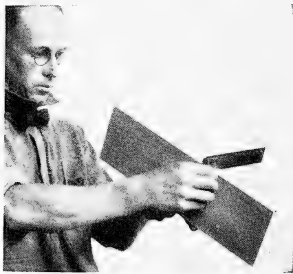
FIG. 61. Testing edge with try-square.
