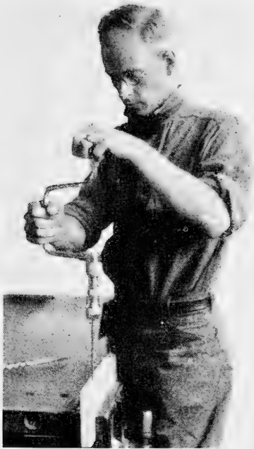
FIG. 33. Correct method of using auger bit.
