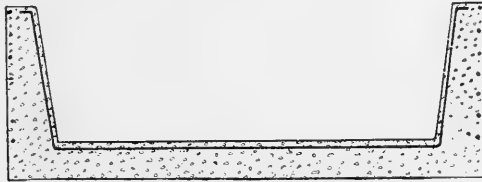
FIG. 167-a. Cross-section of finished tank.
