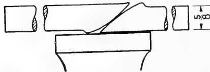
FIG. 204. Position of pieces when welding.
