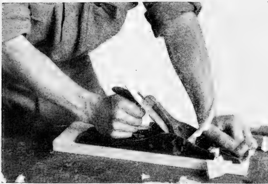
FIG. 59. Correct way of holding the plane.
