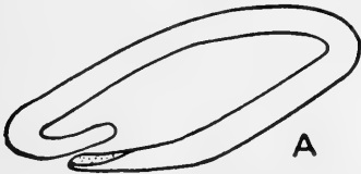
FIG. 233. Preparing the weld.
