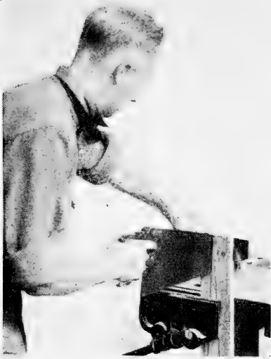
FIG. 18. Correct position when using rip-saw.
