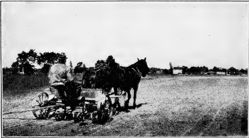
FIG. 13.—Planting seed with a special beet drill.
