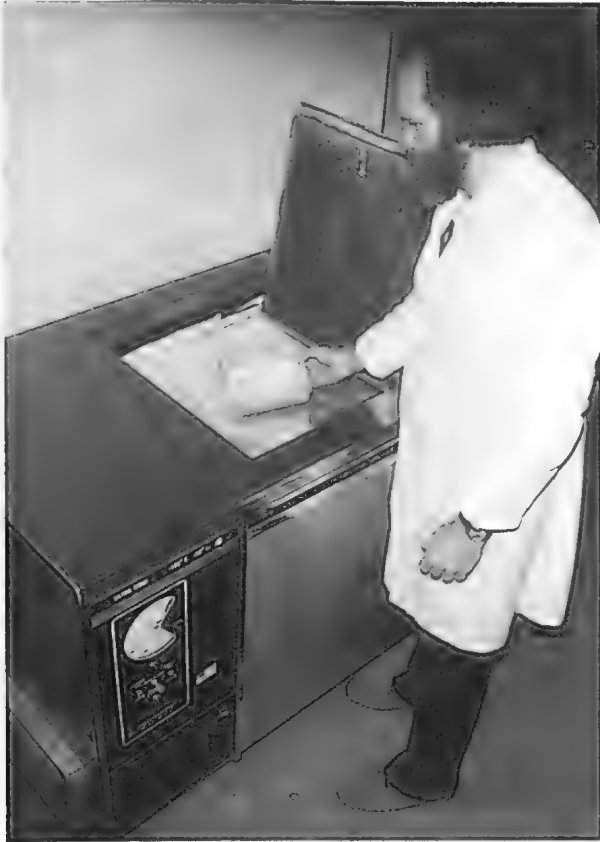
Figure 14.7 Storage of tissues in an ultra-cold storage unit at the South Australian Museum. Such units maintain sufficiently low temperatures to preserve proteins for both short-term analysis and long-term storage.
