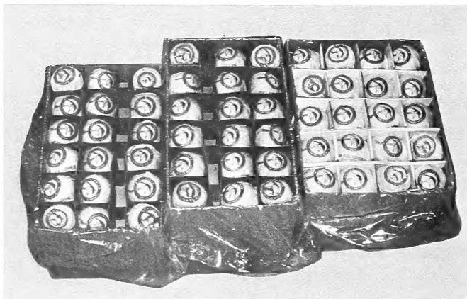
FIGURE 3.—Boxes used for Golden Delicious apples, count size 80, in test shipments from Washington to New York City, March–April 1966: Left , 50- by 30-cm. (FTHSC) three-layer box holding 54 apples; center , 50- by 30-cm. (FTHSC) four-layer box holding 72 apples; right , control C (FTHSC) four-layer box holding 80 apples. Note space dividers, or air cells, in 50- by 30-cm. boxes.
