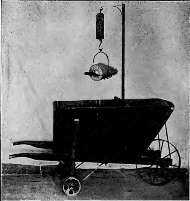
FIG. 51.—The "meal cart" used for weighing concentrates for the individual cows in the herd. (Ottawa Station.)
