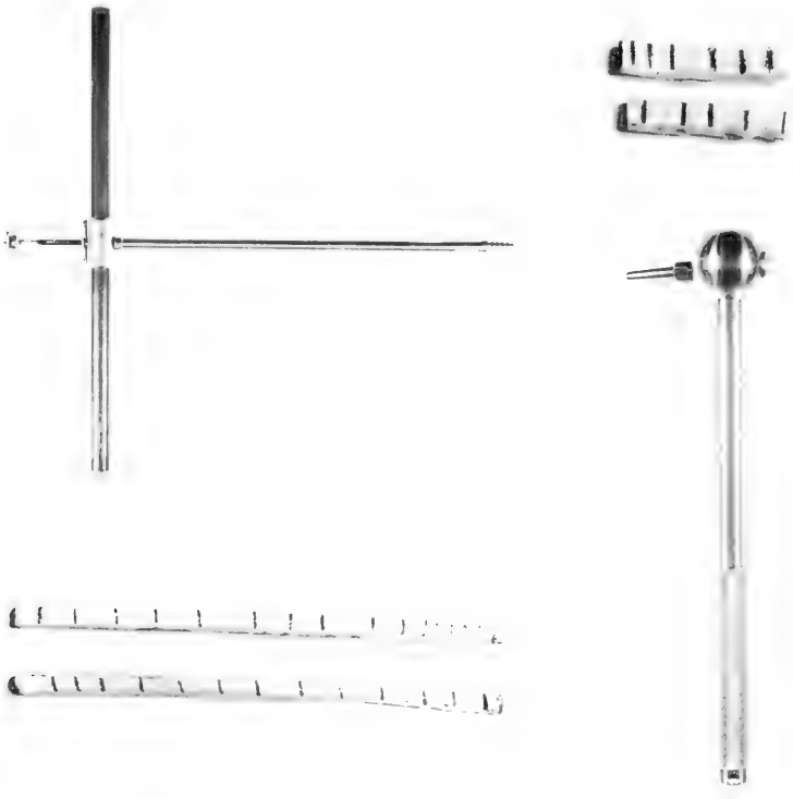
FIGURE 2. The increment borer (left) and the increment hammer (right) are tools used by the arborist or forester to obtain cores from the wood of standing trees. The cores obtained with each have been marked with ink to make the widths of the annual rings more evident. In each instance, the upper core's most recent annual rings are closely spaced, indicating a slow growth rate; the rings of the lower cores are widely spaced, indicating the rapid growth of healthy trees.
