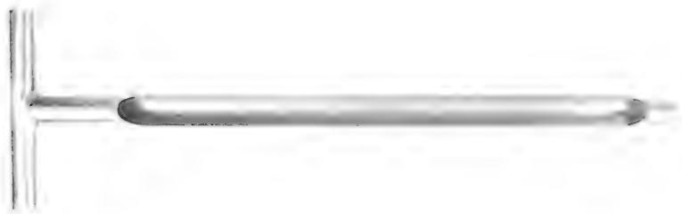
FIGURE 3. The soil-profile tube is a handy tool for removing cores from the upper 10–14 inches of soil. Many properties of the soil can be observed by examining such cores.
