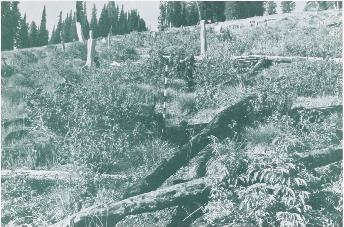
Figure 4—An example of class I roughness (1.2) due to the many downed logs and tall stumps; boulders and rock outcroppings can create the same effect. This site occurs at 7,700 feet in elevation with a 20-degree azimuth and a 55 percent slope. These site conditions can produce snow pressures of 1,210 pounds/foot.
