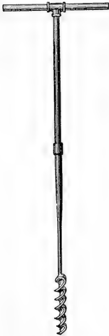
FIG. 3.—Soil Auger Made by Welding a Three-foot Length of Wrought Iron Gas-pipe onto the Shank of a 1½-inch Wood Auger. Additional lengths may be added as desired.
