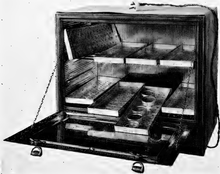
FIG. 21.—A Gasoline Stove Oven, Galvanized Iron Trays, and Tin Dishes for Drying Soil Samples.
