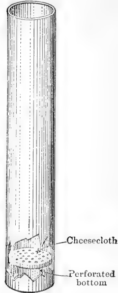
FIG. 13.—Brass Cylinder Used to Measure the Water-holding Capacity of Soils.
