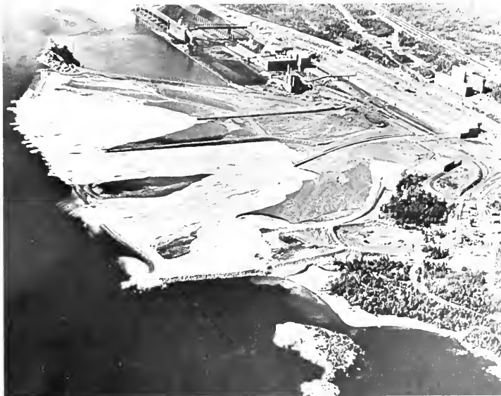
Aerial photo of Reserve Mining Company's Silver Bay (Minnesota) plant on Lake Superior. During a normal day's operation, some 67,000 tons of taconite tailings—which contain asbestos fibers—are dumped into the lake.
