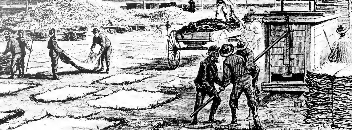
An 1874 woodcut showing a typical railroad hide yard. Staked hides dry in the sun. Three men in the foreground operate a hide press. Stacked at the right is a
