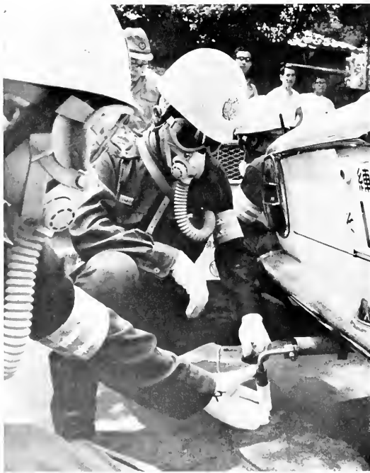
Japanese policemen measure CO content of auto exhaust in downtown Tokyo. Emissions from autos and other man-made sources account for only about 6.5% of the CO produced on earth (United Press International Photo)
