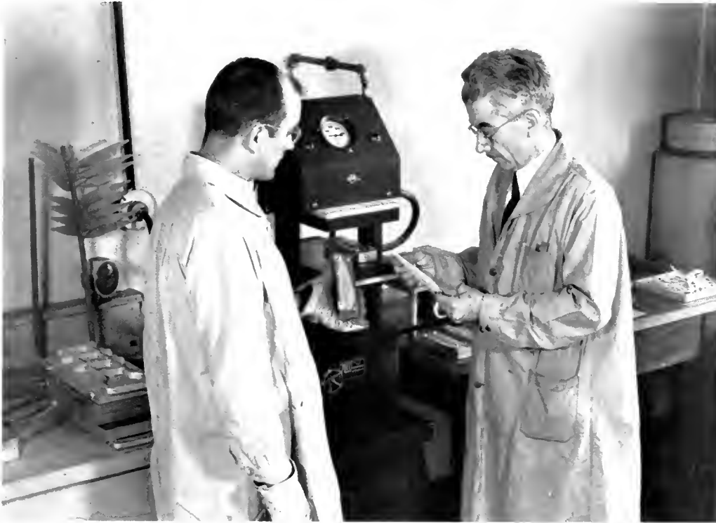
Frank Boryca (FM1947-1972), left, and Emil Sella (1898-1965, FM1938-1961) shown in 1947 while making plastic leaf models with hydraulic press. Large leaves, such as those of cabbage, were made of wax in plaster molds. Smaller leaves were made of plastic in metal dies. Boryca was a preparator in the Department of Botany, Sella's position was curator of exhibits for Botany. BB0328
