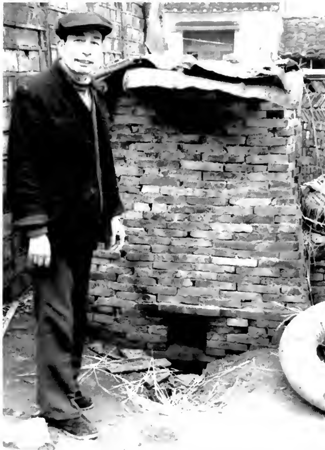
6. COMMUNAL KILN at Lumu for firing cricket jars. The pipe at right is for blowing air into kiln. Photo: Ho C.M.
