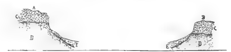
COMPARATIVE SECTIONAL SKETCH OF THE CLIFFS OF THE LIMPIA (A) AND HOPPELLOS MOUNTAINS (B) A. Trachyte Rocks. B. Yellow Sandstone. C. Debris.
