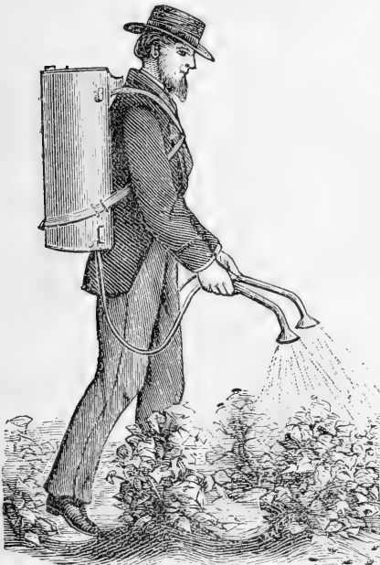
Gray's Improved Sprinkler, for the use of Paris Green water.
