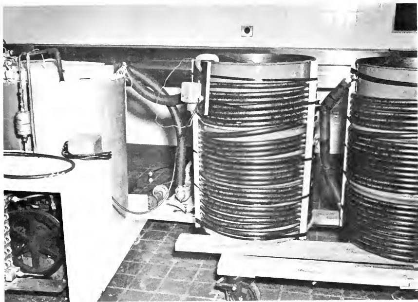
FIGURE 1.—Arrangement of the brine chiller (on the left); the pump is (on the floor) for circulating the chilled brine through the cooling coils shown wrapped around the uninsulated holding tanks.
