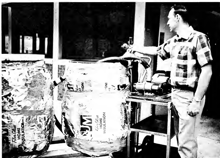
FIGURE 2.—Arrangement of the Moyno pump for recirculating chilled brine in the holding tank (on the left) and the CO 2 cylinder (in the back) and attached CO 2 flow meter (being adjusted by the worker).
