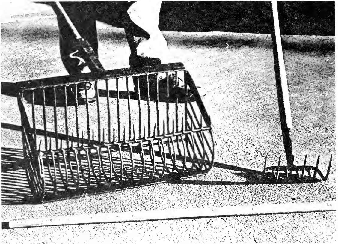
FIGURE 1.—Differences between the bull rake (left) and pea digger (right) in number and spacing of teeth, and head size and mass.
