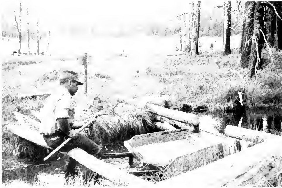
FIGURE 15.—The South Creek fry trap and the method of counting young fish.
