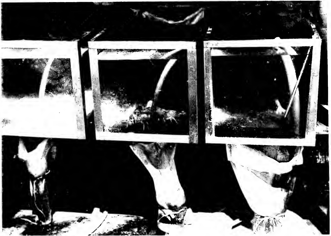
FIGURE 1.—Aquariums used in rearing experiments, showing plankton netting attached to collecting jar to catch larvae and eggs in runoff.
