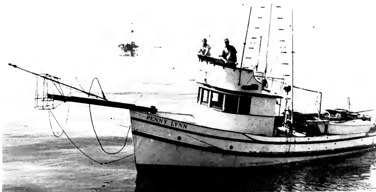
Fishing operations research small swordfish vessel equipped with harpoon gear, now turning to basking shark fishery in off-season.
