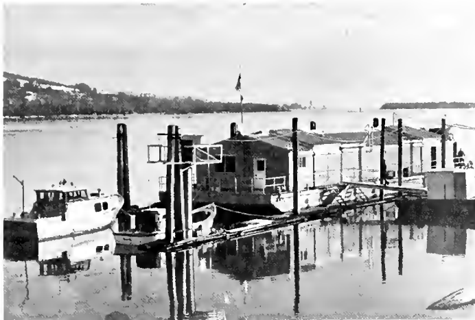
FIGURE 34.—The biological field station at Prescott, Oreg., houses biological and chemical laboratories plus two “wet” laboratories. Each wet lab has twenty-two 50-gallon tanks that can be individually supplied with heated or cooled water from the Columbia River.
