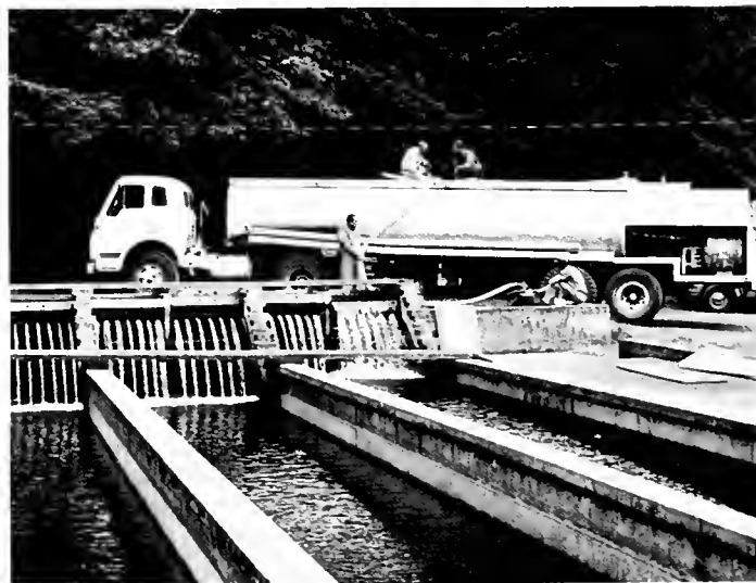
FIGURE 40.—Truck used to transport fingerlings around dams. The 5,000-gallon tank truck has a refrigeration-aeration system and filter. Capacity is 400,000 fish, 2½-inches long.
