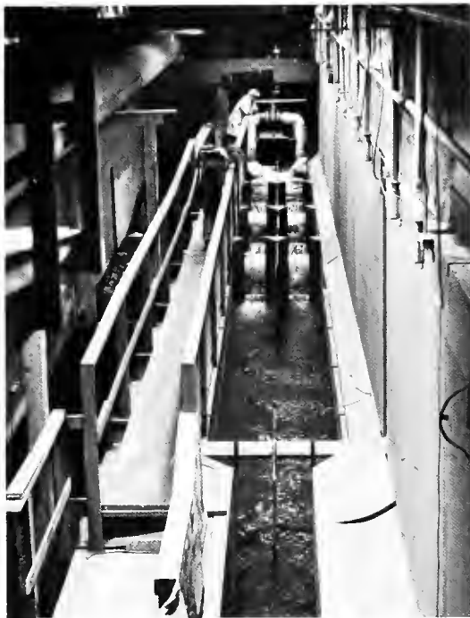
FIGURE 25.—Observers follow fish through the temperature test channels at Bonneville Dam. Heated or cooled water can be supplied to either channel by regulating valves from heaters and chillers without changing hydraulic conditions in either channel.
