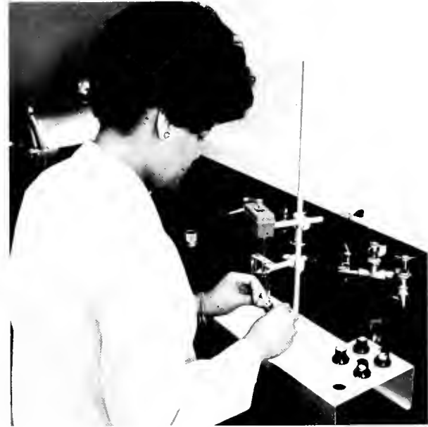
FIGURE 47.—Technician preparing density gradients for ultracentrifugation to isolate enzymes.
