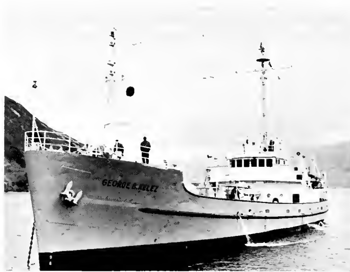
FIGURE 4.—The George B. Kelez , a converted military cargo ship, is 176 feet long, has a cruising speed of 11 knots, and carries 6 scientists and a crew of 14. The vessel was named for a scientist from the Biological Laboratory who lost his life in a plane crash while on duty in Alaska in 1954.
