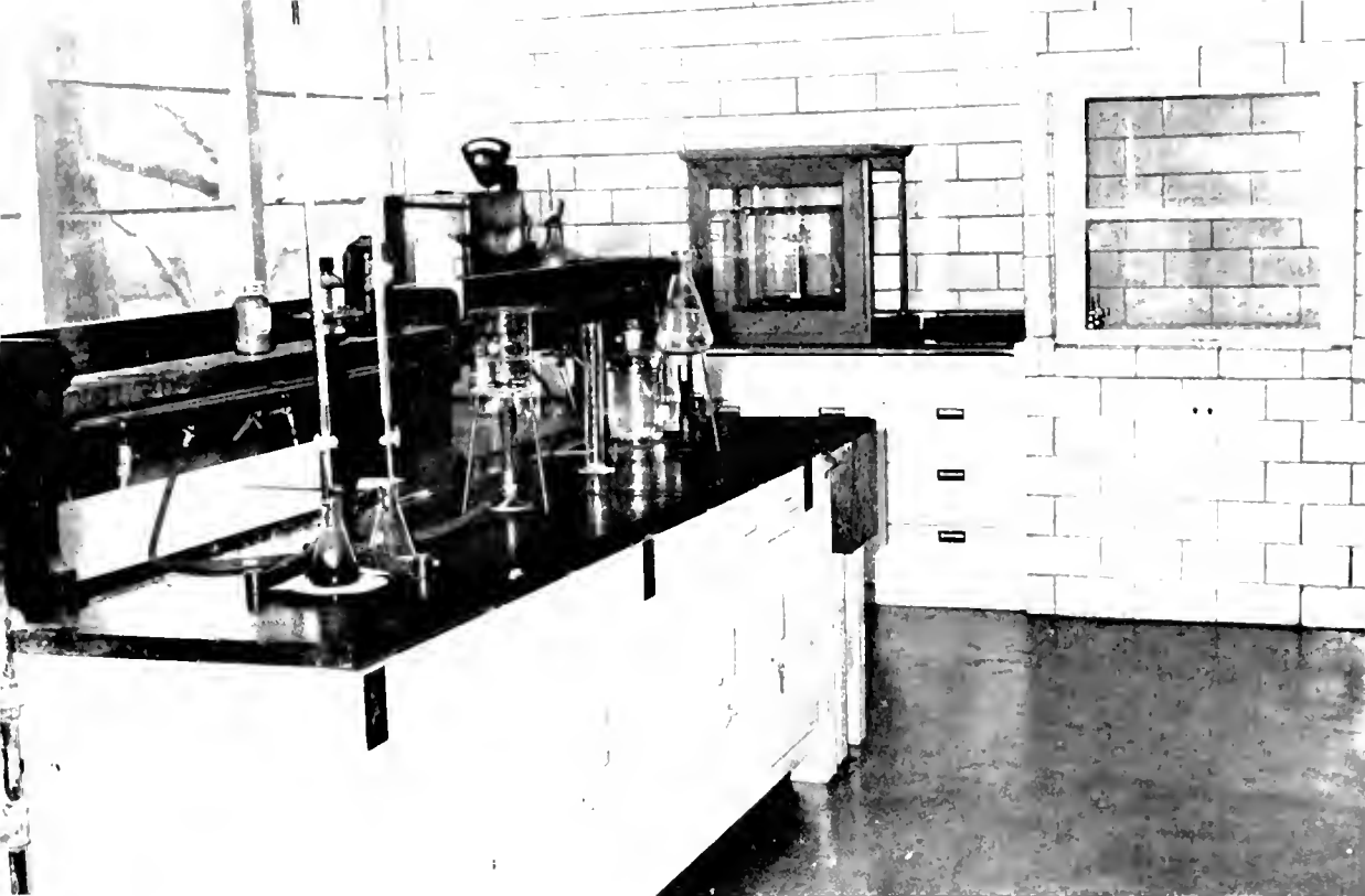
Close-up of chemistry table showing the hot and cold-water, gas, and air connections. In the background are the analytical balance and fume hood
