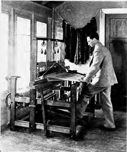
Demonstrating the Flying Shuttle on the Loom. There Are No Really Efficient Domestic Looms on the Market. The Flying Shuttle Was Added to This Loom on the Homestead. With This Attachment, a Yard of Cloth Is Readily Woven in an Hour. The Suit Worn by the Demonstrator Was a Hand-spun Twill Woven on This Loom and Made-up by a Local Tailor.
