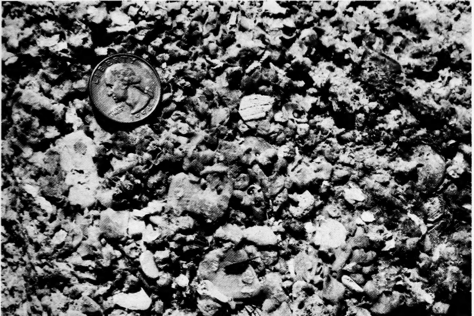
FIG. 3. Surface of coquinooid limestone in the Anastasia Formation showing broken and abraded mollusk shells. Diameter of coin is 2.4 cm.
