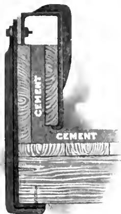
Fig. 1. Wittbold Bench Clamp. simple problem even to those not possessed of recognized mechanical ability. E. H. Hunt, 76 Wabash avenue, Chicago, is placing on the market these accessories, which comprise the outfit for building benches under the Wittbold system of construction, that has proved to be one of the most simple, as well as successful, systems yet followed, and which entails the least expense. We are pleased to present illustrations of the work in detail, and to describe the method of construction.
