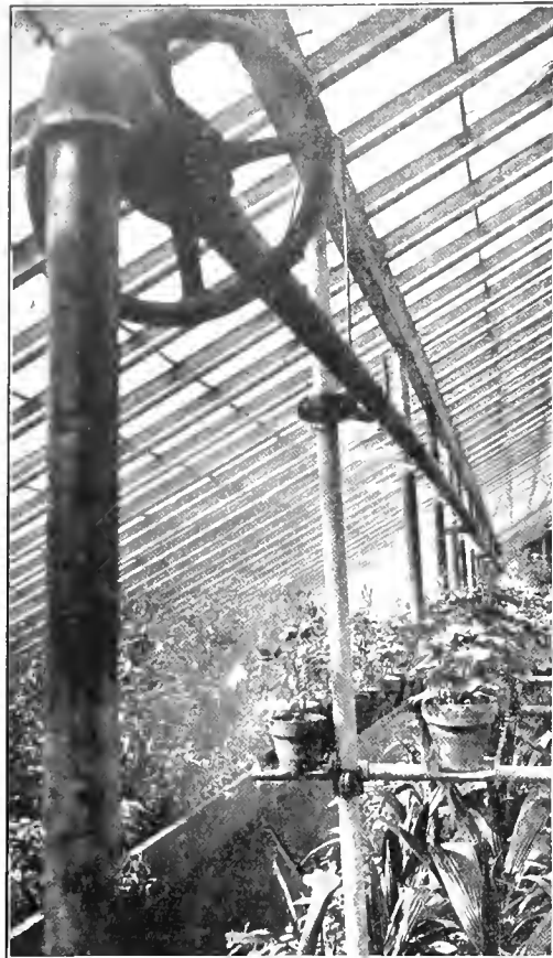
Wittbold Watering Device in Operation upon a Side Bench—The Showering Effect is Plainly Seen in the Photograph
