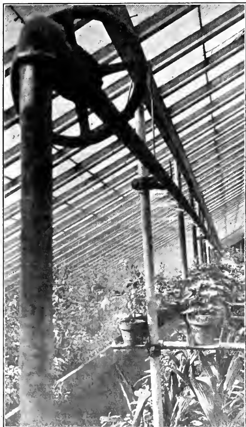
Withhold Watering Device in Operation upon a Side Bench. The Showering Effect is Plainly Seen in the Photograph.
