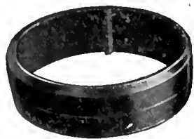
The cast iron nipple is milled with a slight slant from the front edges to the center so that the more you pull up the short tie rods, the tighter you set the nipples.
