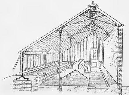
Fig. 65. THREE-QUARTER SPAN GREENHOUSE.
