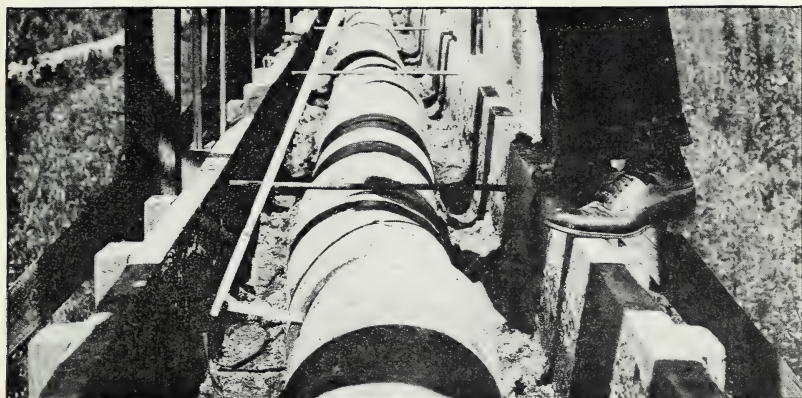
FIG. 2.—12-INCH CLAY TILE AS LAID TO DETERMINE THE EFFECT OF IRREGULAR JOINTS ON THE COEFFICIENT OF ROUGHNESS.
