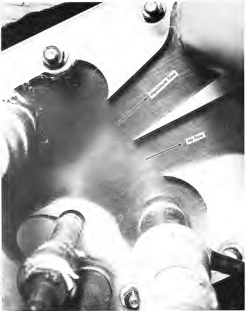
Figure 30. Flow pattern through the amplifier with 0.267 gpm of control flow.
