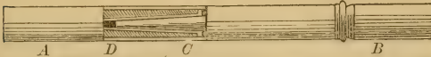
Fig. 41.—Dowelled Ferrule: A , end of middle joint; B , end of tip; C , dowel; D , its socket.
