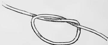
Fig. 20.—The ordinary knot.
