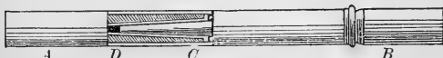
Fig. 41.—Dowelled Ferrule: A , end of middle joint; B , end of tip; C , dowel; D , its socket.
