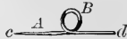
Fig. 77.— A , body of pin; B , loop made in middle of pin; c and d , ends of pin.
