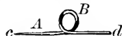
Fig. 77.—A, body of pin; B, loop made in middle of pin; c and d, ends of pin.
