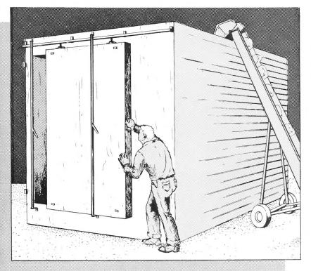
This insulated cooler is 11 feet 2 inches high, 18 feet 11 inches long, and 10 feet wide. It will cool about 250 bushels of fruit at one time.
