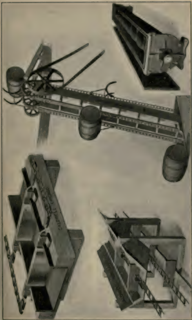
The illustrations at the left show two styles of scraper flight conveyors. At the right are a barrel elevator and a spiral flight conveyor.
