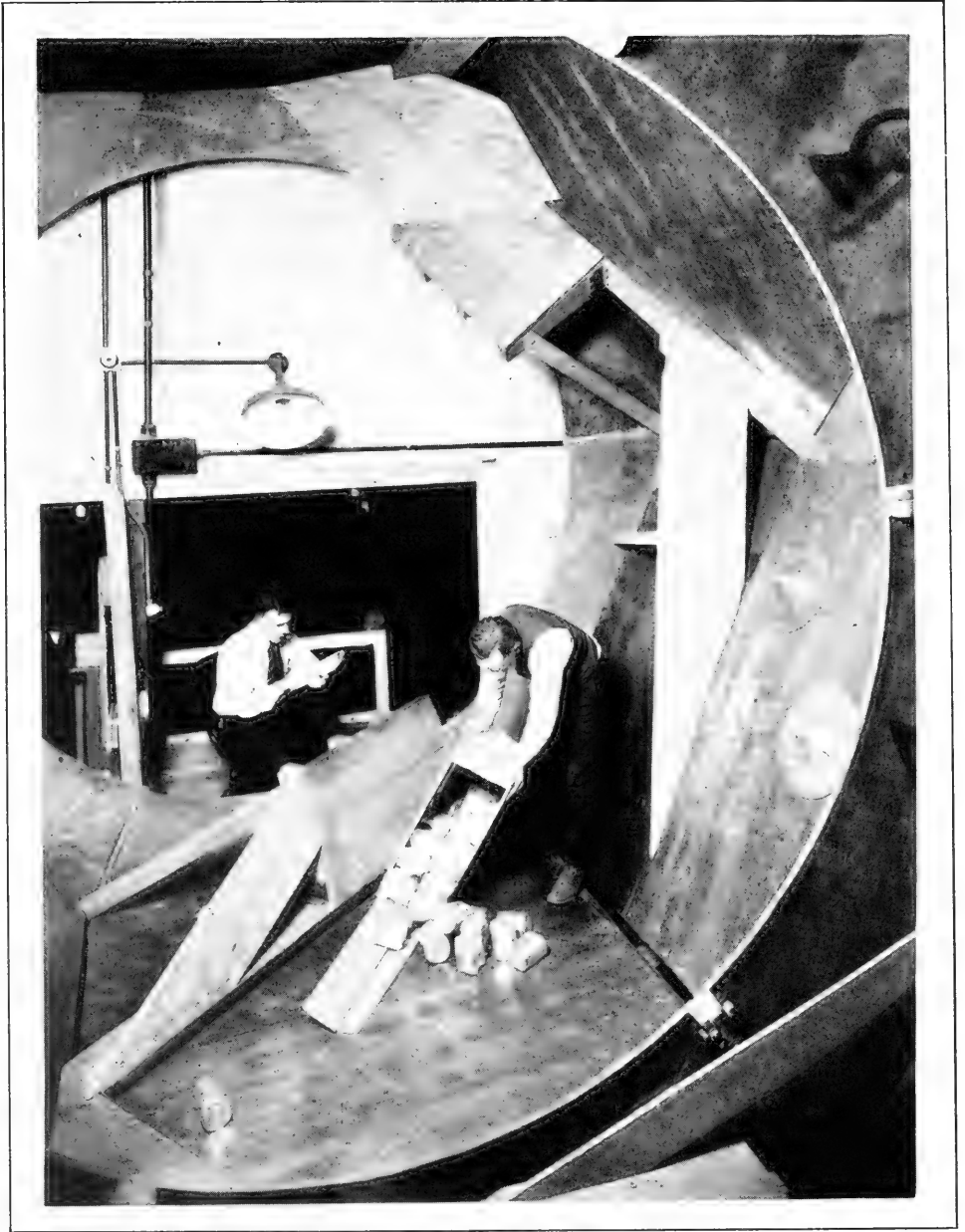
BOX TESTING IN THE BIG TUMBLING DRUM—A LABORATORY DEVICE FOR QUICKLY DETERMINING BOX OR CRATE WEAKNESSES
