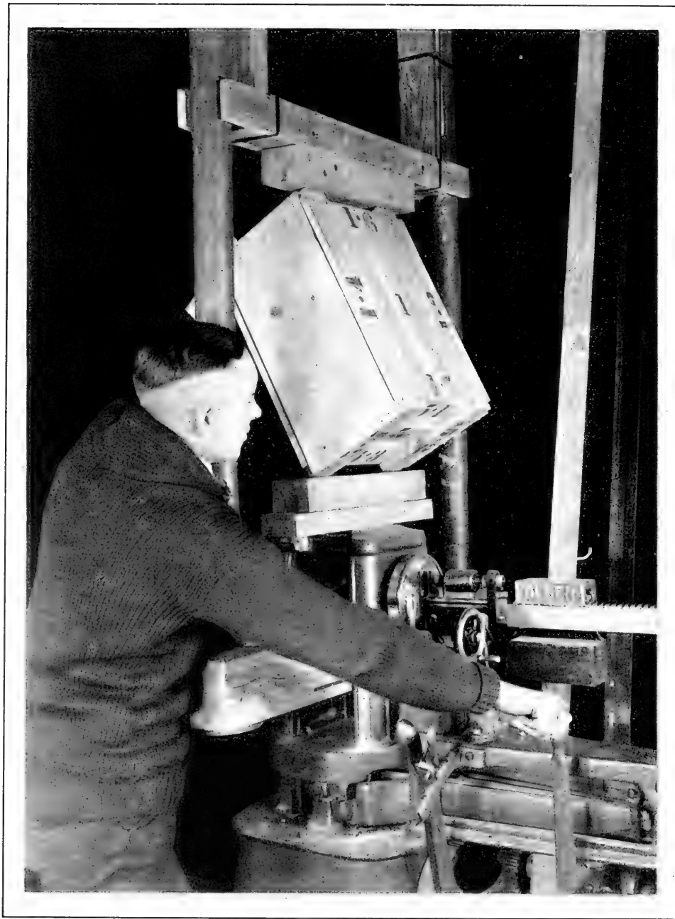
COOPERATIVE BOX WORK—A STUDY OF DIAGONAL COMPRESSION
