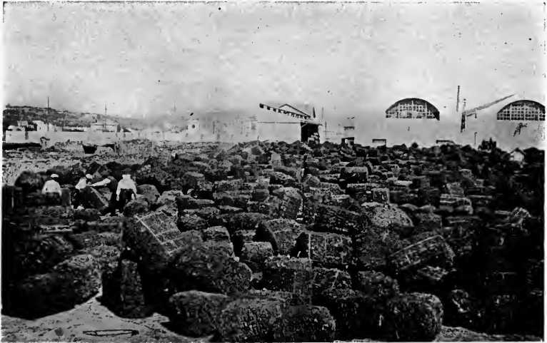
FIG. 120.—Baled cork scraps at a cork factory. Used principally for insulation at refrigerating plants.
