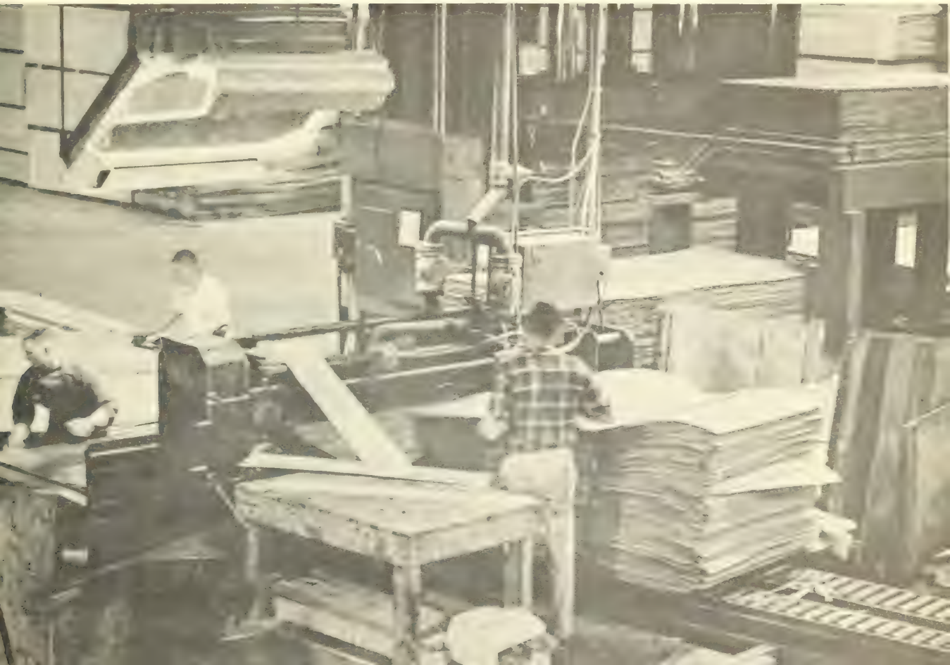
Glue spreading, Van-Evan Plywood Company, Missoula. Photo: Charles R. Lockard.
