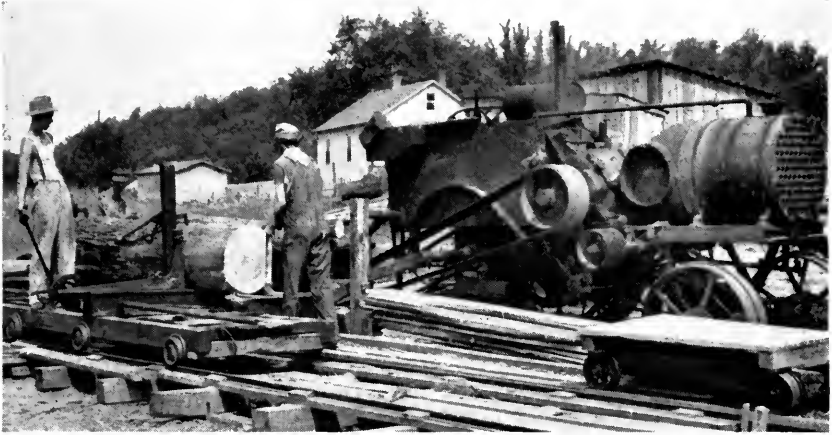
Sawmills that produce less than 50,000 board feet of lumber annually are generally poorly equipped and capable of producing only low-quality lumber. Most of this lumber is used locally on farms. (Fig. 27)
