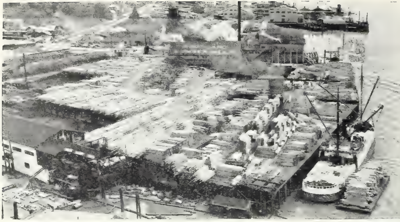
FIGURE 27.—Large sawmill on the Willamette River. In the foreground is a veneer plant; at the extreme left are seen the cores remaining after logs and bolts are peeled
