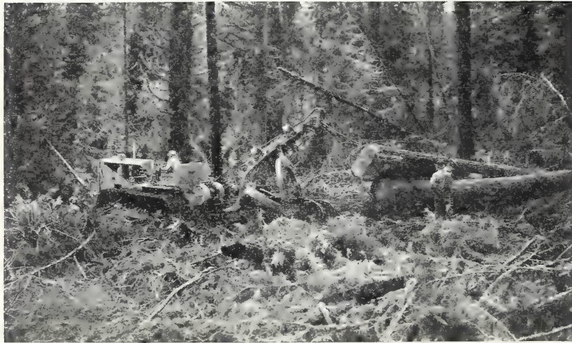
FIGURE 23.—Logging Douglas fir with tractor and arch in the Oregon Coast Range. Use of this type of equipment is increasing in the spruce-hemlock and Douglas-fir types of western Washington and western Oregon and is causing significant changes in management of these types
