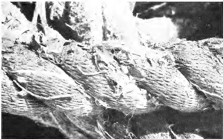
Figure 7. Polypropylene line with numerous tube worms and small horse mussels concentrated along lays. A light fouling of red algae is also present.
