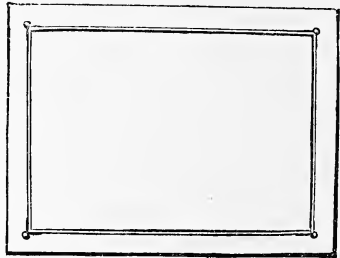
FIG. 11. BOTTOM OF PORTABLE AQUARIUM, showing Grooving for Glass and Zinc Moulding.
