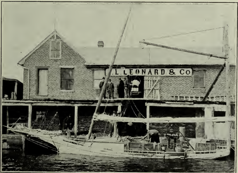
FIG. 2.—UNLOADING OYSTERS BY MEANS OF A CRANE OPERATED BY A DONKEY ENGINE IN THE SMALL BUILDING AT THE RIGHT.
