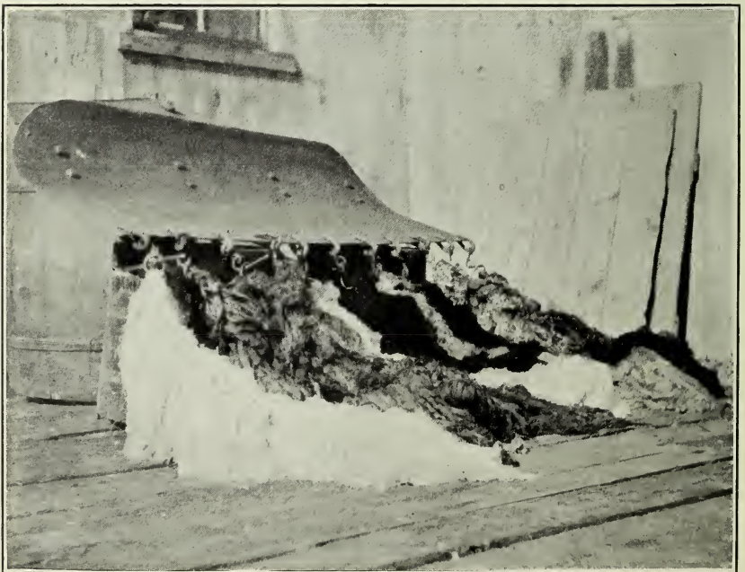
FIG. 2.—"DISH-PAN" FORM OF STAR MOP, USED IN LONG ISLAND SOUND.
