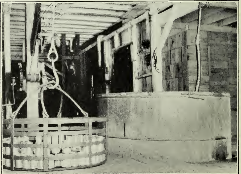
FIG. 2.—BASKET OF CANNED OYSTERS, AFTER HAVING BEEN "PROCESSED," READY TO BE LOWERED INTO THE "COOLER," AT RIGHT, WHERE RUNNING WATER IS PASSED ABOUT THE CANS.
