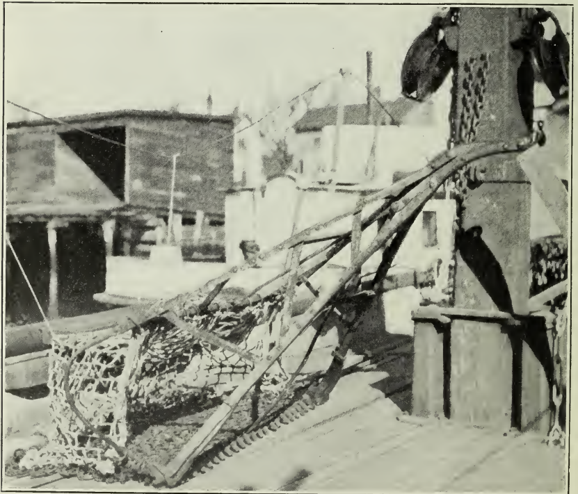
FIG. 2.—MACHINE-HOISTED DREDGE USED IN TAKING OYSTERS.
