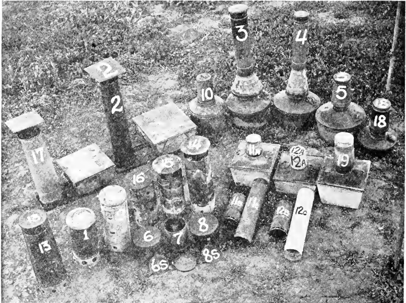
Fig. 15.—Names of the heaters tested: 1. Pomona. 2. Kittle. 3. Scheu Jumbo Cone Louvre. 4. Scheu Baby Cone Louvre. 5. Scheu Double Stack. 6. Bolton. 6s. Bolton (with spider). 7. Troutman. 8. Canco. 8s Canco (with spider). 9. Diamond. 10A. Dunn (10 in the illustration). 10C. Dunn (with 30-inch stack; not shown). 11A. Citrus, 9-gal. low stack. 11B. Citrus, 9-gal. medium stack. 11C. Citrus, 9-gal. high stack. 12A. Citrus, 6-gal. low stack. 12B. Citrus 6-gal. medium stack. 12C. Citrus, 6-gal. high stack. 13. Karr. 14. Jessen (large). 15. Jessen (medium). 16. Jessen (small). 17. Low Delivery. 18. Baby Double Stack. 19. Citrus Gas Flame. (From Agr. Exp. Sta. Bul. 442.)
