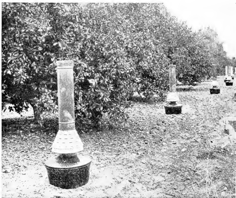
Fig. 10.—Citrus orchard banked with heaters on the windward side; one large capacity heater per tree.
