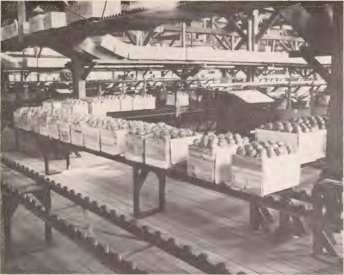
FIGURE 32.—Interior of a packing house in the Río Negro. Note conveyors, rotary bin grading machinery, and other mechanical labor-saving devices common to American packing houses. (Courtesy of Great Southern Railway.)
