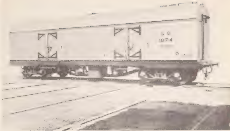
FIGURE 41.—Refrigerator car used by the Buenos Aires Pacifico Railway for transporting grapes from the San Juan-Mendoza area to Buenos Aires. (Courtesy of Buenos Aires Pacifico Railway.)
