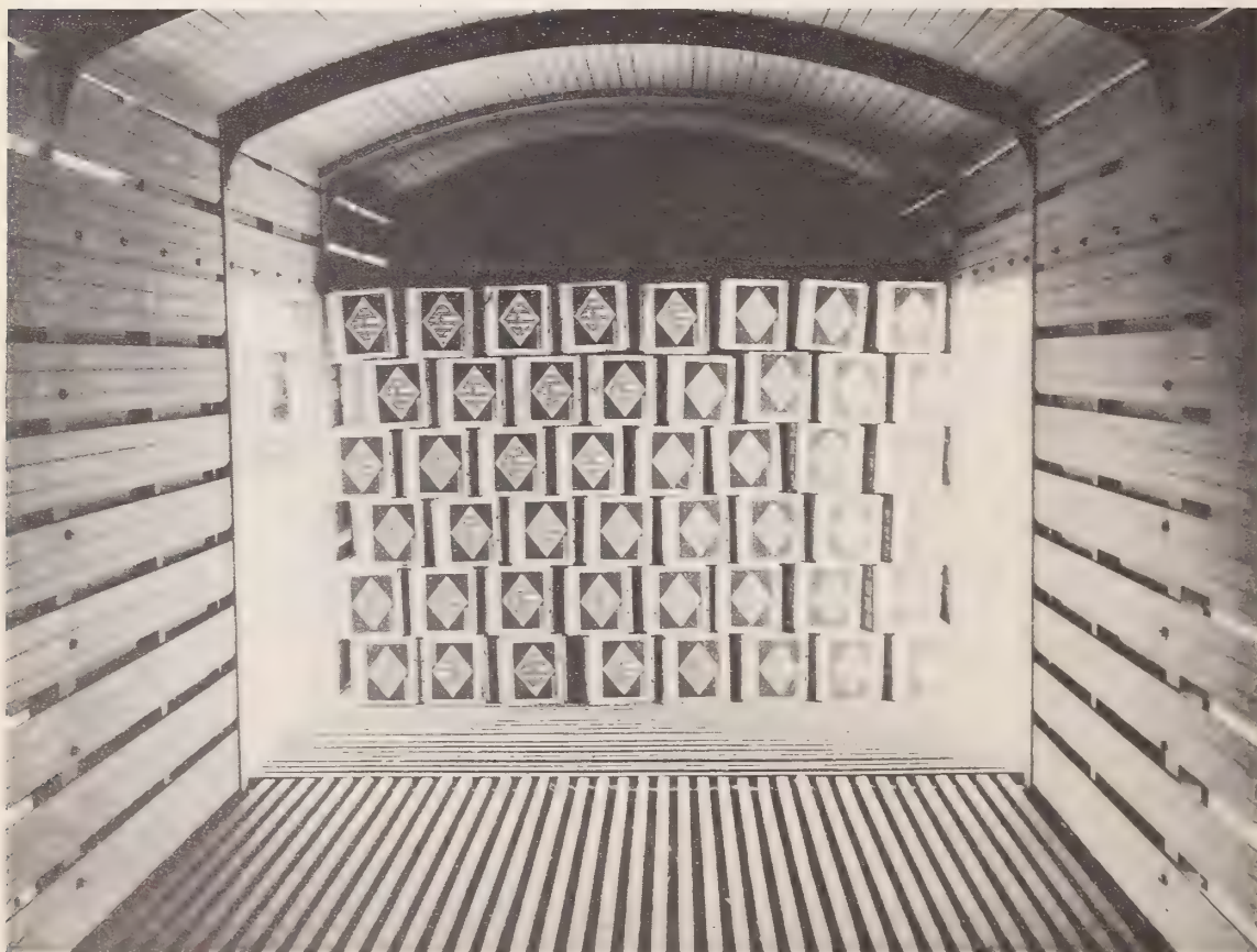
FIGURE 34.—Ventilated car used in transporting apples and pears from the Río Negro Valley. This type of construction gives excellent ventilation and permits surprisingly rapid cooling. It has a capacity of about 900 boxes. (Courtesy of Great Southern Railway.)
