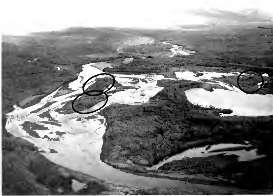
Figure 65. Penny River mined area looking upstream. Note the flooded conditions within the disturbed area, and the overburden piles in the center of the site (circled on photograph).
